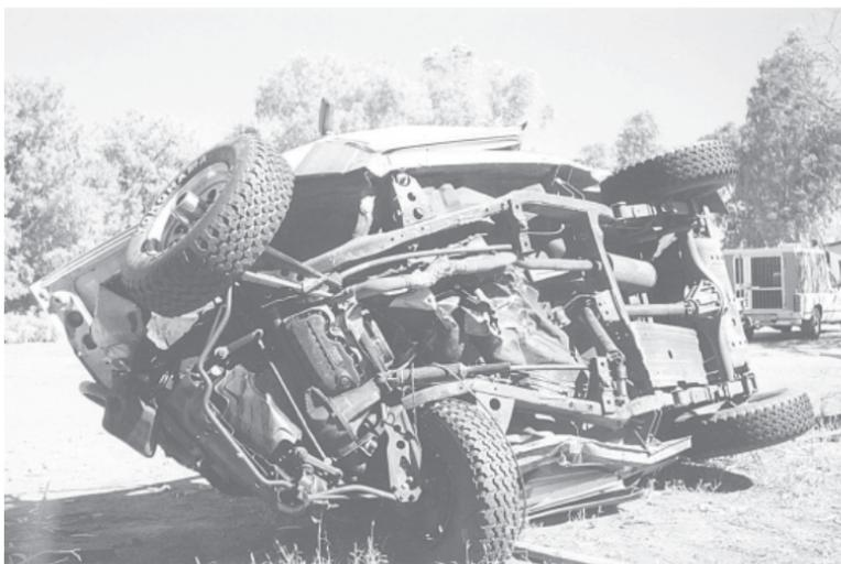
*The underneath shows the solid chassis members of this small truck buckled under the force of collision with the much heavier vehicle, at a combined speed of 110 mph (180 kph).*
