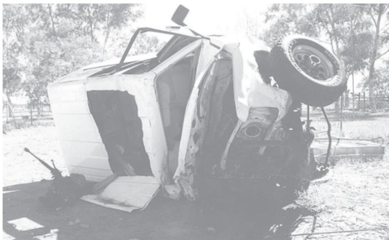
*The wrecked vehicle in an Alice Springs salvage yard, in the same position as after the accident, resting on the driver’s side. The roof is still peeled back where it was cut open to extract the driver, several hours after the impact.*
